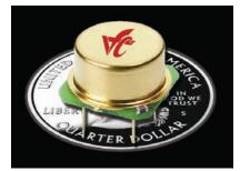
10°C above the maximum operating temperature and held steady, producing minimal frequency variation due to external ambient temperature changes; 5 to 10-ppb temperature stability is commonly available.
